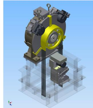
Figure 4 Rope Gripper pre-mounted on PMAC machine
